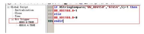
Script: if HDW150input string and the string "87654" is equal, HDX180.01; HDX180.00 is not equal.
