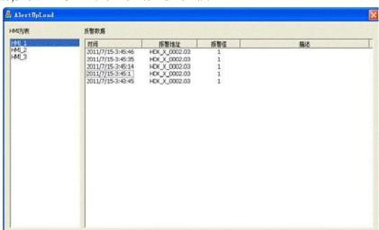
Click the name of HMI can check the alarm data.
