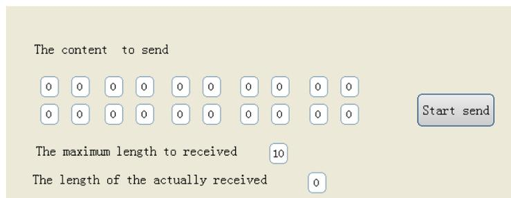
In this example ,it will read 10 data from the serial port into ReadNum register.
