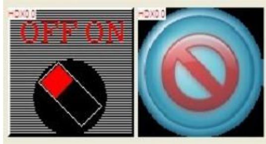
Figure 3-11 bit switch with bitmap appearance
